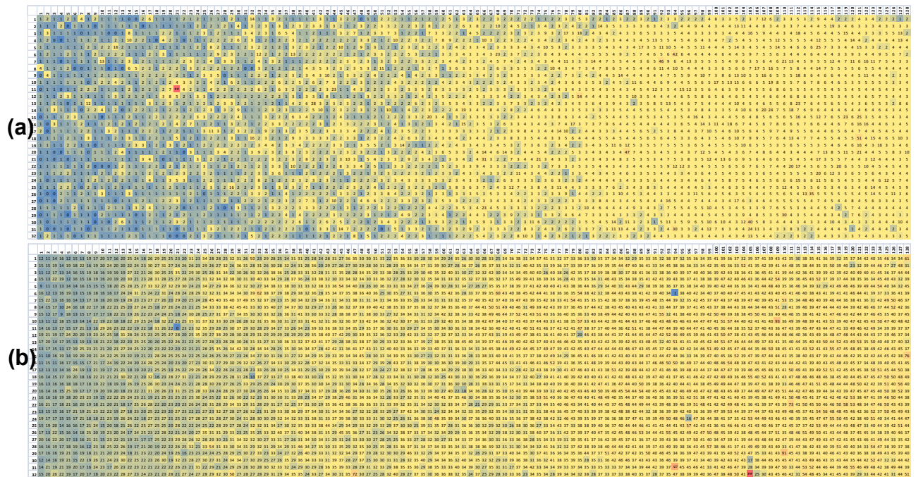
Figure 5. Performance maps of all 4096 pixels of a 32 x 128 InGaAsP/InP (1.06 \mu\text{m} ) GmAPD FPA operating with an excess bias of 2.25 V at 248 K. (a) Dark current density (in kHz) for all pixels shows just 1 high DCR pixel. (b) Photon detection efficiency (in %) for all pixels is reported only for photons hitting the active regions since a microlens array was not present. Two pixels exhibit spurious (high) PDE measurements. Overall pixel operability is >99.9%.
